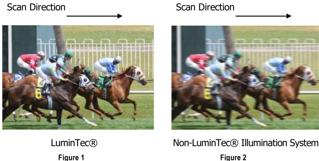
In Figure 1, notice that blurring does not occur with LuminTec Lighting because the pixel columns are frozen by the Strobe. In Figure 2, the fence blurs horizontally because the pixel column is moving during capture, which degrades the overall image. With LuminTec® the effects of the scanning movement are eliminated.
